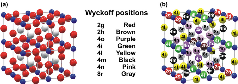
Fig. 1. (a) Copper nitride (2 × 2 × 2) super-cell. Cu and N atoms are shown as red and blue spheres respectively, while vacancies are shown as gray spheres. (b) Cu and vacancy Wyckoff positions are color coded (For interpretation of the references to color in this figure legend, the reader is referred to the web version of the article).
